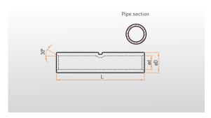
Note: Not recommended for use in copper conductors, in order to avoid galvanic couple.
